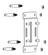
4 Install the bracket to the pre-installed plate
