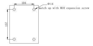
3 Fix the pre-installed plate
