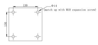
③ Fix the pre-installed plate
