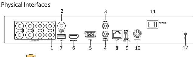
The rear panel of DP-1204/1216Q-F1/N provide 4/16 video input interfaces.
