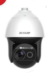
Dunlop 4K series DP-22DF8836I5V-AELW smart PTZ dome cameras are able to capture high quality images in dim light environment with its laser IR light, which can reach up to 500m IR distance. Embedded with 1/1.9" progressive scan CMOS chip makes true WDR (120dB) and 8MP real-time resolution possible. With the 36X optical zoom Day/Night lens, the camera offers more details over expansive areas.
